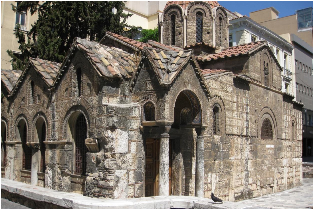
Figure 90: Exonarthex with propylon and south façade of Panagia Kapnikarea in Athens. The two visible bays of the exonarthex (left) are replicated to the north. The exonarthex with several saddle roofs, dual windows in the center, and single windows at the edges mirrors the configuration of the porch of the south basilica of Qal 'at Sim 'ān.
